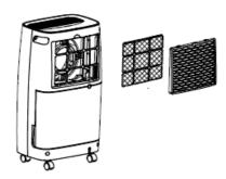
Gently vacuum clean the filter to remove any dirt. If the filter is exceptionally dirty, wash it with warm water and a mild cleanser and dry thoroughly.
