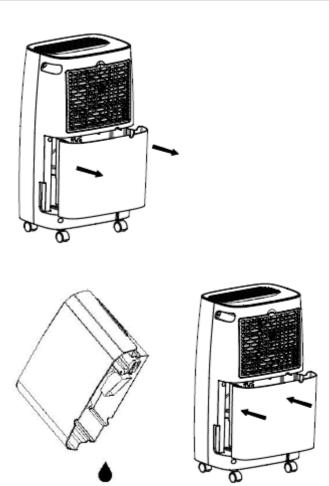
**Note:** Do not remove the float from the water tank. The water full sensor will no longer be able to detect the water level correctly without the float and water may leak from the water tank.
