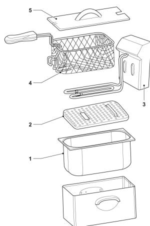
The deep fryer has a 'cold zone' at the bottom of the appliance. The 'cold zone' is a zone where larger food particles sink and the lower temperature keeps them from being burnt by the oil or the liquid fat. Deep fryers with a 'cold zone' have many advantages, but also require special attention. Deep fryers with a 'cold zone' are sensitive to water as the heating element is immersed in oil or liquid fat. Water can get in touch with the oil or the liquid fat due to various causes:
